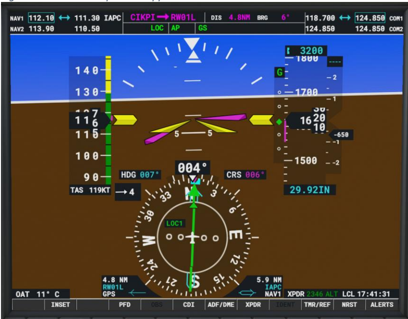
Figure 75 - Final Example - ILS Approach PFD
