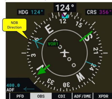
Figure 58 - Tracking to the NDB
