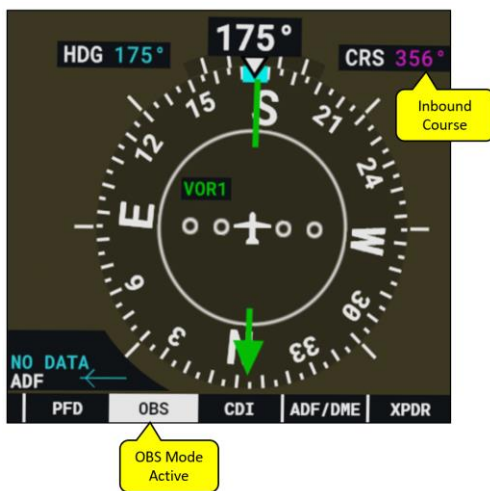
Figure 58 - Tracking to the NDB
