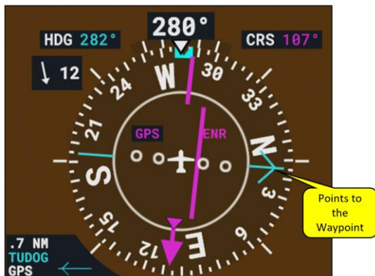
Figure 45 - GPS Hold Pattern HSI
