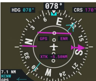
Figure 8 - Using OBS & DIRECT-TO For Runway Alignment
