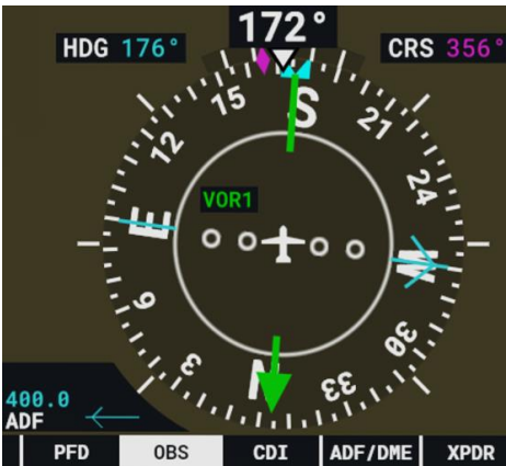
Figure 59 - NDB Example - Turning to the Outbound Course
