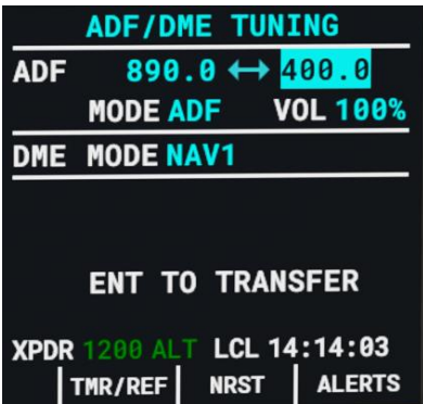
Figure 57 - NDB Example - Tuning an NDB
